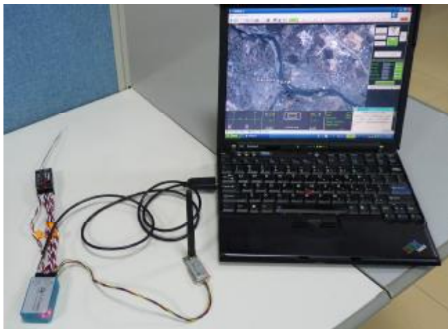
Figure 1: At your ground Station, the signals from your RC Transmitter is sent to the RC Receiver which is connected to your computer via the FY-3ZT Remote Adapter.
