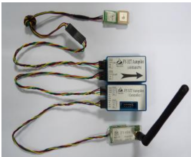
Figure 2: On the aircraft, the radio modem controls all flight parameters. No RC receiver is installed in your aircraft.
