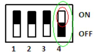
**Step 2:** Move Dip Switch No. 4 to 'ON' position.
