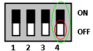
**Note:** when the DIP Switch NO.4 is in the ON position, the FY-31AP will record the neutral point for each time you switch the mode from **Mode 1: Deactivated Mode to Mode 2: Stabilized mode**.
