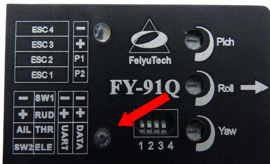
The GPS connection status & vibration level is indicated by the Red LED Flashing:
