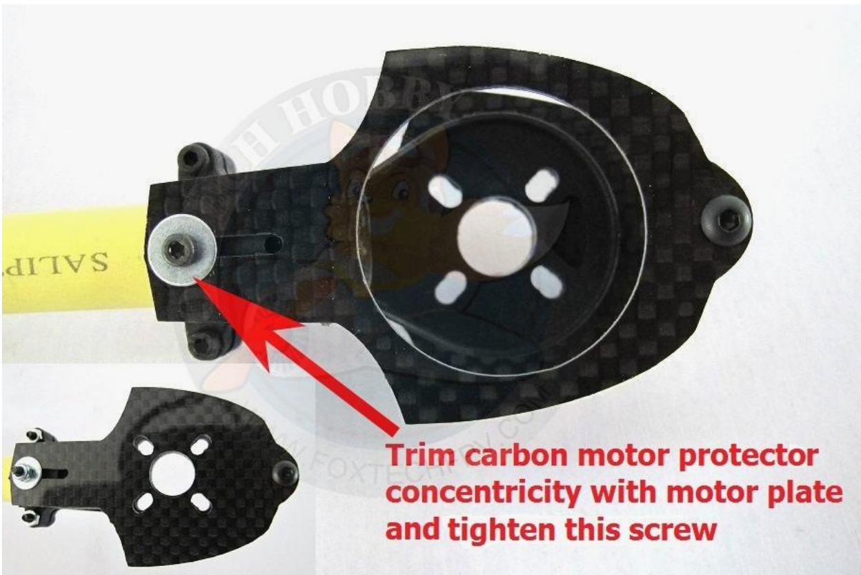
Assemble Motor Seat on Frame Arm.
