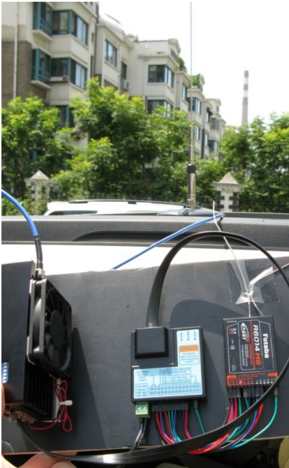
The picture above shows the car antenna installation. The RD6014 needs to be fixed on the inside glass of the car.
