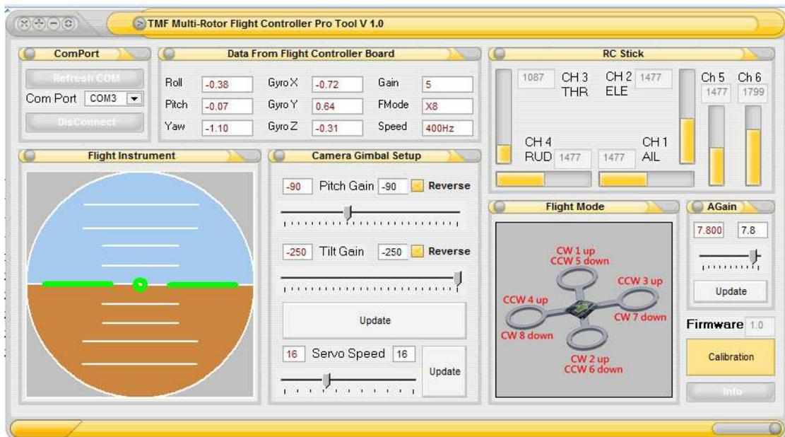
This below group will show 3-axis attitude, 3-axis gyro rate, flight gain, flight mode, and PWM ESC frequency data.
