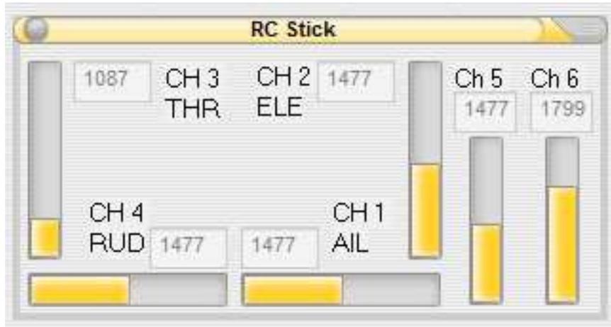
This below group will show the auxiliary gain, if move the RC stick, copter attitude overshoot(usually in big frame over 50cm motor to motor), it means RC stick and attitude coupling control gain is too big, you can reduce this gain value(6.4~8.0).
