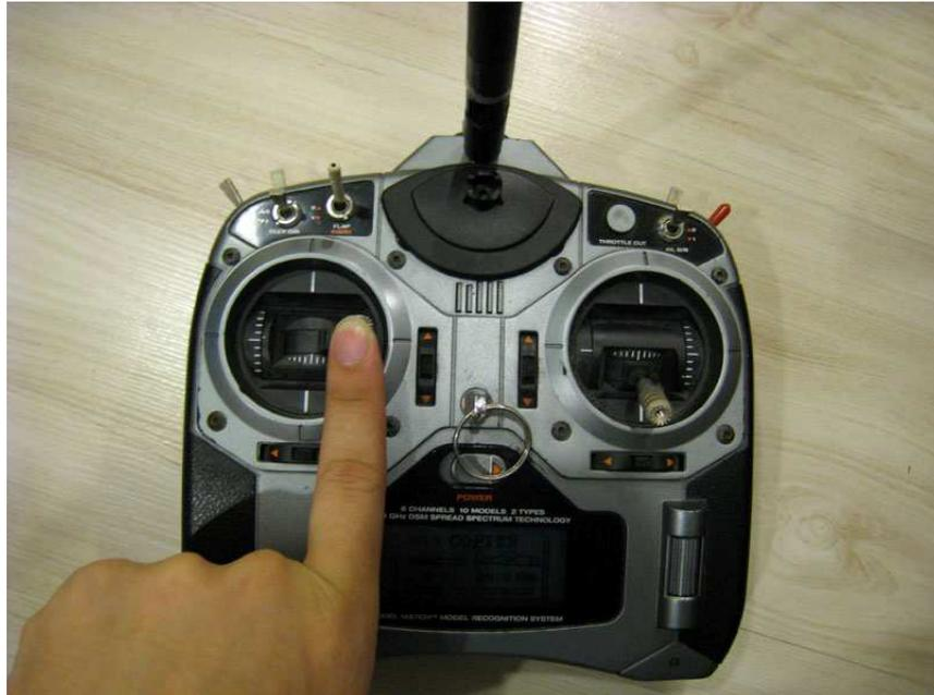
Stop your motor; move the throttle down and the rudder to the left.
