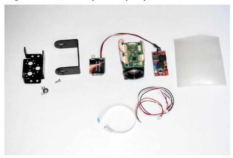
This picture shows zoom cam, its controller, universal v-reg, strong aluminum pan/tilt and clear heat shrink. Pan/tilt and v-reg are optional.
