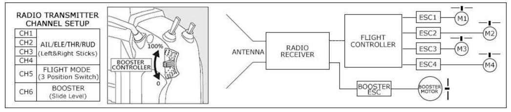
The Sbus/PPM connection requires a radio receiver with both Sbus/PPM and PWM output same time, and the booster ESC must to be plugged in radio receiver directly, and assign a transmitter CH to 'Slide level' to control the booster power.
