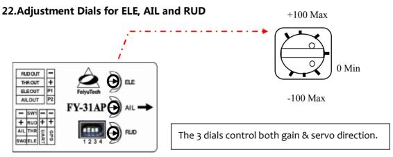
There are 3 adjustment dials on the FY31AP. Each dial controls <u>both</u> gyro gain <u>and</u> servo direction during auto stabilization.
