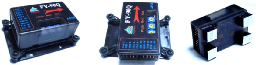
Only the vibration damping pad is enough when the vibration is not so big.
