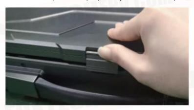
2. Press and hold the computer's rear power-on button to turn on the computer
