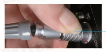
When unplugging the cable, use your fingers to push back the position shown in the figure above to unplug the cable.
