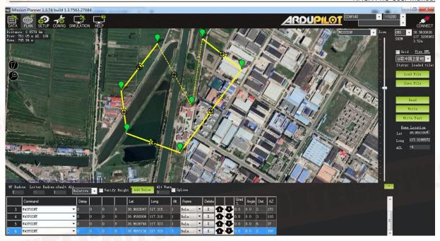
The main explanation here is the mission planning function of the MP ground control station, but the waypoint planning concepts of other ground control stations are actually very similar.
