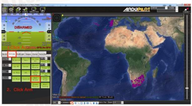
ARM Successfully: The propeller will spin up at idle speed to remind that it has been successfully unlocked.
