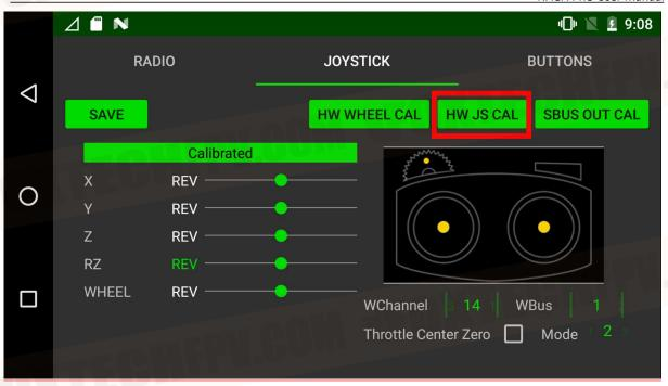
To calibrate the joystick, click start calibration, and perform hardware joystick calibration according to the joystick arrow and the prompt on the right.
