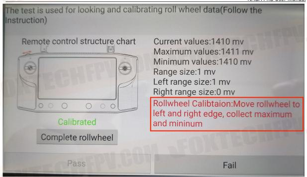
• After the calibration is completed, you can set the Sbus channel of the rollwheel and the Sbus1 or Sbus2 to be used at the position marked with the red frame. The output of Sbus1 is the same as the output of the joystick, and the rollwheel can be set to channels 5-16, and on Sbus2, the rollwheel can be set to channels 1-16
