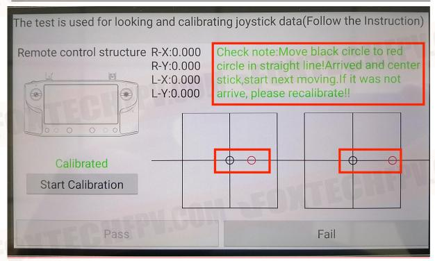
After the joystick calibration is completed. It will prompt that the test is passed, click the
