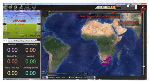
• Data Transmission Connection Method: usually use USB to connect the data link of the ground station you need to select the corresponding COM port, and set the baud rate on the right side to 57600. For WIFI or Bluetooth to connect the data link of the ground station, select the corresponding device from the device list and input the IP address in the device list. For specific parameters, please refer to your data link instructions first.
