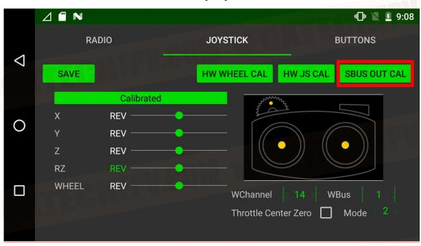
• Follow the remote controller moving steps on the right to move the joystick to each corresponding position.
