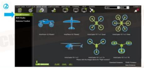
After connecting, follow the instruction and messages to install firmware. When it shows "Download Completed", unplug and replug the USB cable.
