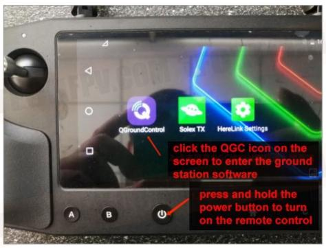
Enter the ground station software and wait for the aircraft to automatically connect.
