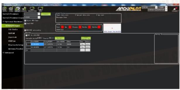
Enter the latitude and longitude of the known fixed station and the measured height of the RTK antenna relative to the ground at the position in the figure below, and then click the use button.
