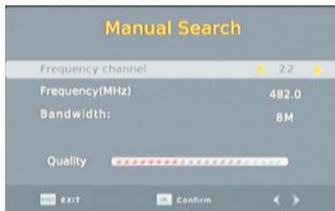
The menu shows frequency channel, frequency, bandwidth, quality. Press OK to enter Channel search processing.
