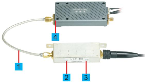
1. Wave filter line , SMA Male to SMA Male connection line
