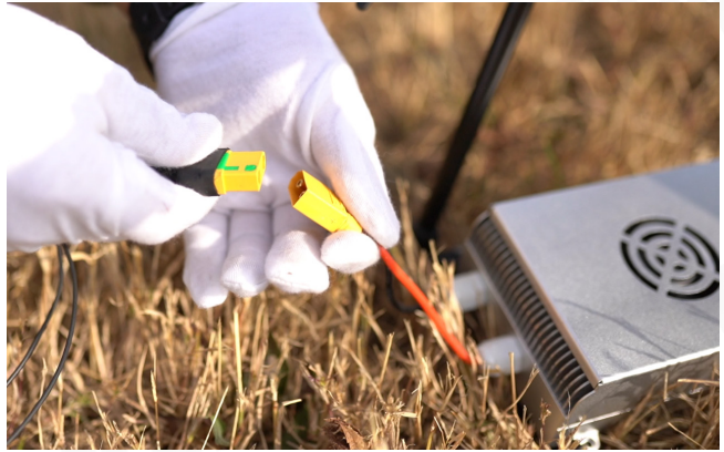
2. Connect the cable jack-plug to the onboard power input port.
