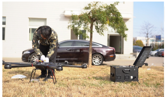
4. Connect onboard power output end to the drone battery interface.
