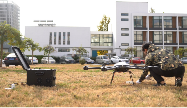
1. Pull out the cable 3~5m, suitable for the drone
