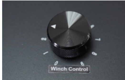
Winch control knob- Max.6.5,excessive tension will lead to overload failure,need to reset by main switch.
