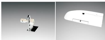
2. Fix the quick connector to the control horn, and then glue it.
