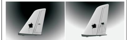
4.Install the servo of the V-tail and then glue the control horn and slip the pushrod as the above pictures show.
