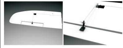
3.Slip the pushrod for the main wing into the hole, and then tighten the screw.
