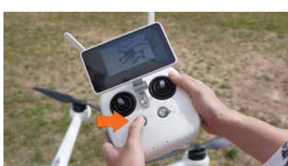
11. Turn on the remote controller.
