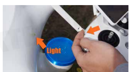
12. Toggle the flight mode switch on the remote controller back and forth until the aircraft status indicator turns yellow.
