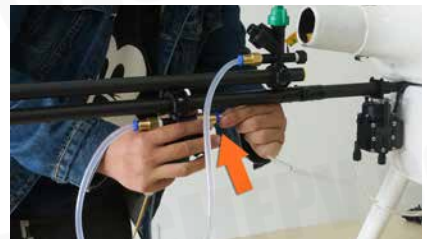
3. Connect water pipe.
