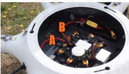
10. Note: if use two batteries, connect one battery to A cable, the other to B cable.
