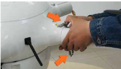
7. Fix the arms and lock the hooks.
