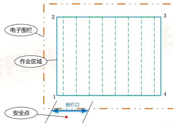
★ If switch to the manual mode when operation in Auto, “polygonal” fence will not disappear. If switch to “Return flight” (including break point), and then switch to “manual mode” when operation in Auto, “polygonal” electronic fence will disappear.
