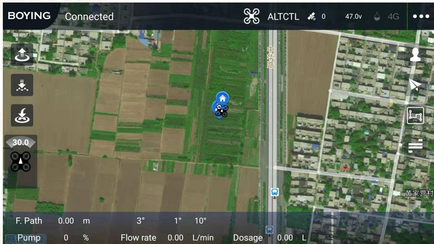
Installing and turn on the obstacle avoidance radar. When radar detects the obstacle, the ground station displays the distance between the aircraft and the obstacle. The obstacle avoidance hover mode is triggered when the aircraft approaches the obstacle. At this time, the obstacle avoidance hover mode can only be cancelled by pulling the pitch joystick backward. The automatic obstacle avoidance function is applicable in both manual and automatic modes.
