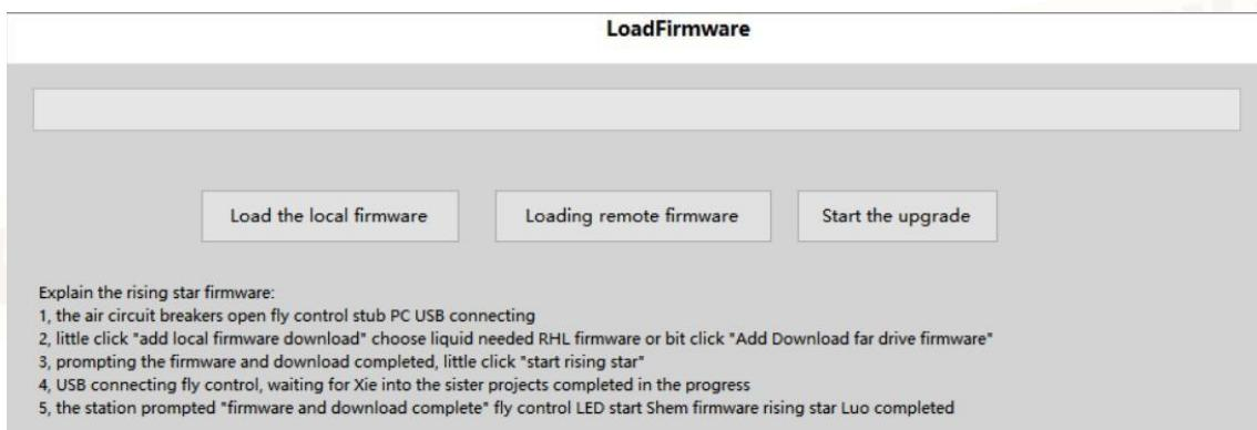
Click "Load local firmware", select pre-update firmware (file ending with .byaero), confirm and click "Start upgrade", connect USB cable to the main control, wait for about 10 seconds, the progress bar is completed, the main control indicator lights up, the firmware upgrade is finished.
