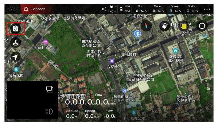
**Help point:** Adding point to correct positioning deviation while do second spray works.
