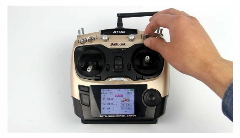
4. Turn the level to switch the 3 modes of Following, Locking and One key return.
