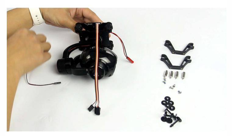
Step 1: Insert the control cable to the right port of gimbal for functions of mode switching, zooming, pitching and 5V output.
