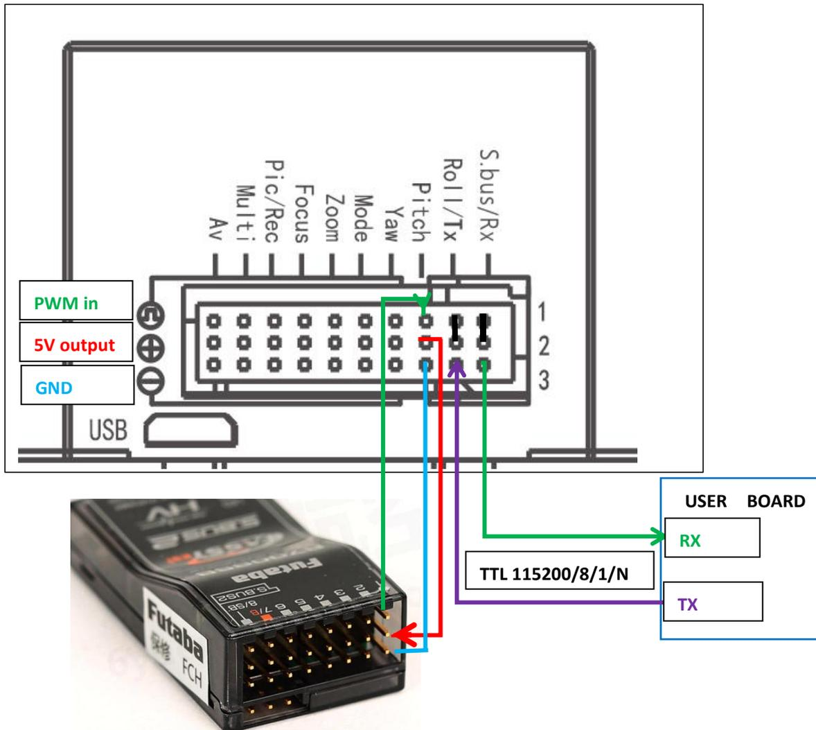
S.bus/Rx : connect to Rx2 for track function.
