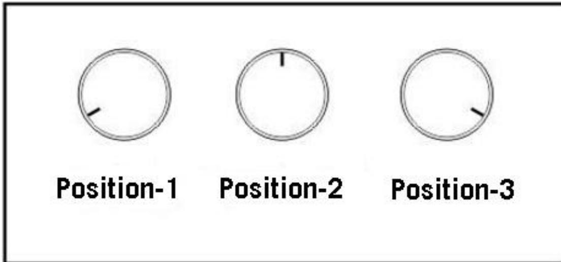
Rotate knob to position-3:low speed lock mode.The gimbal will move at the lowest speed when controlling YAW and PITCH, and gimbal YAW axis will not follow drone flight direction.
