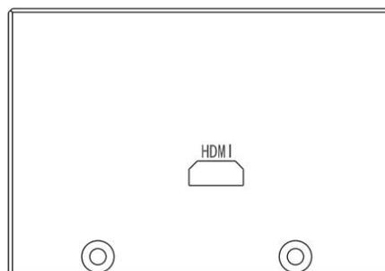
**Notice:HDMI output is 1080P 30FPS,SD card supports max class 10**
