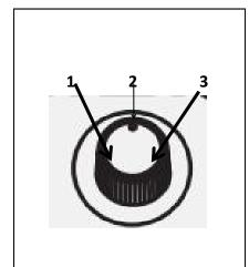
Position 1: lowest speed for pitch and yaw. Position 2: middle speed for pitch and yaw.
