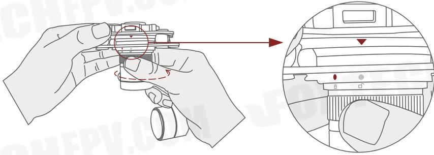
2. Align the white dot (unlock icon) to the red triangle (below unlock button), push the gimbal into the plate completely and then rotate the gimbal camera anticlockwise.
