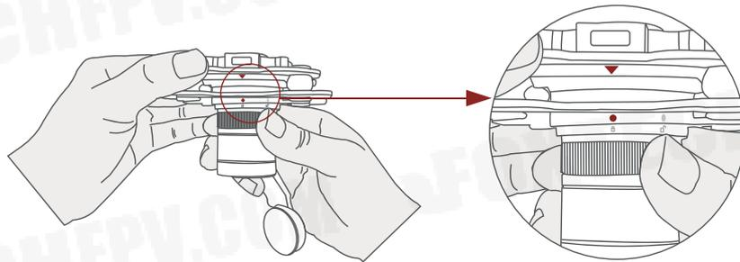
3. When you hear "click" sound (when red dot is aligned to the red triangle) means the gimbal camera and the plate has been locked.
