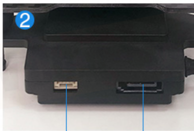
Ethernet Port Can Port
