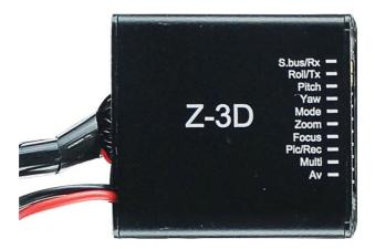
Normally we will control the AOTM via "Multi" channel via controller, please connect it to a 3 gears channel.Flip the channel from low gear to middle gear, then a cursor will appear on the screen, you are able to move the cursor via the controller YAW and PITCH axis(used to control gimbal YAW and PITCH axis).Once you move the cursor to the object you want to track, flip to high gear then the object is locked and will be tracked automatically by the gimbal.
