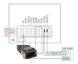
S.bus/Rx: connect to Rx2 for track function.
