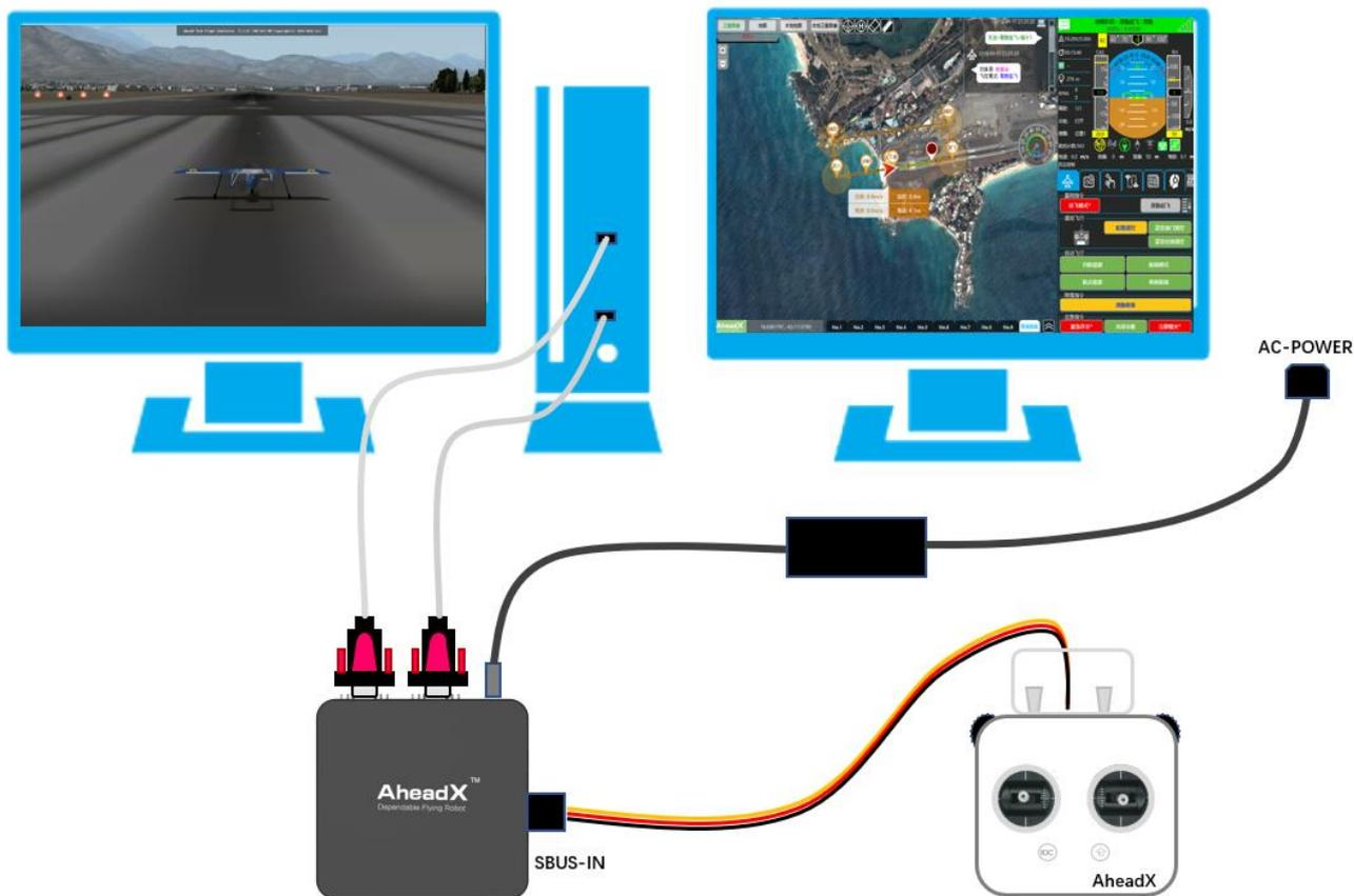
Equipment's COM1 (right side of picture) is connected to the AheadX Space ground station, and COM5 to ASHIL Console software. It is recommended to use Z-TEC 232-to-USB serial cable which you need to install the matching drive.
