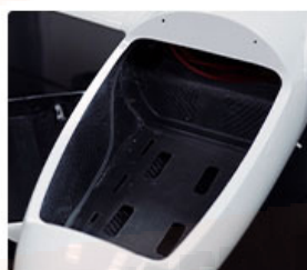
260x150x85mm Battery Compartment
