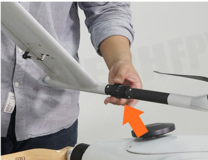
10. Twist the tail part on the arm.
