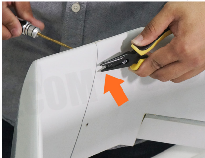
8. Tighten the tail with two screws.
