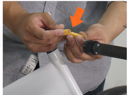
9. Connect the servo cable.
