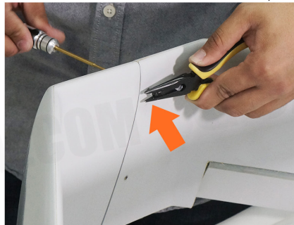
8. Tighten the tail with two screws.
