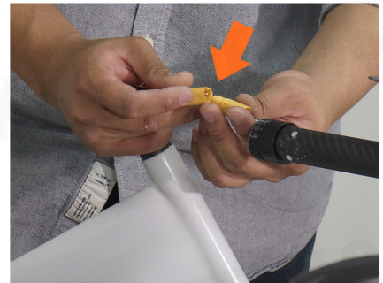
9. Connect the servo cable.
