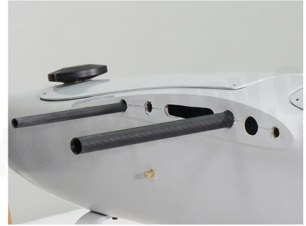
3. Insert the two carbon fiber tubes in the body.
