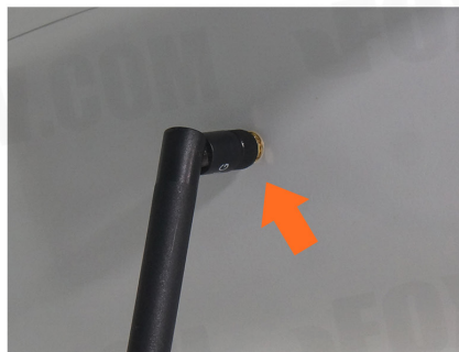
11. Install the receiver antenna.
