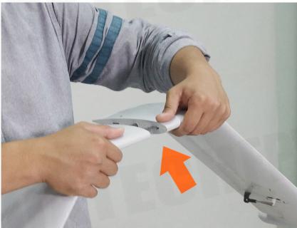
7. Assemble the tail.
