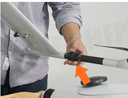
10. Twist the tail part on the arm.
