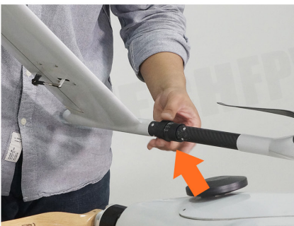
10. Twist the tail part on the arm.
