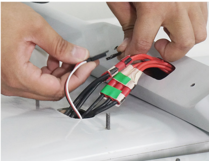
1. Connect the two motor cables and the signal cable.
