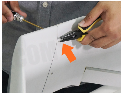
8. Tighten the tail with two screws.
