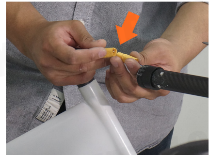
9. Connect the servo cable.
