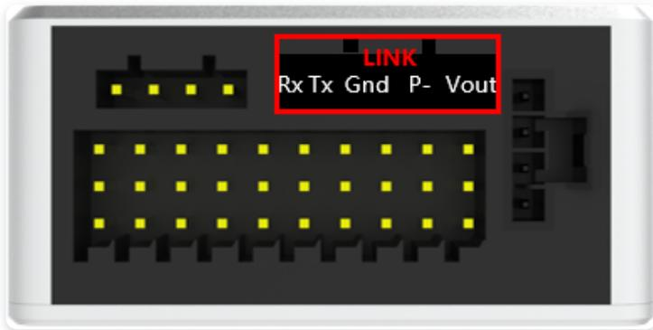
RS232 communication interface, can be directly connected to the AheadX DL900 digital transmission airborne terminal.
