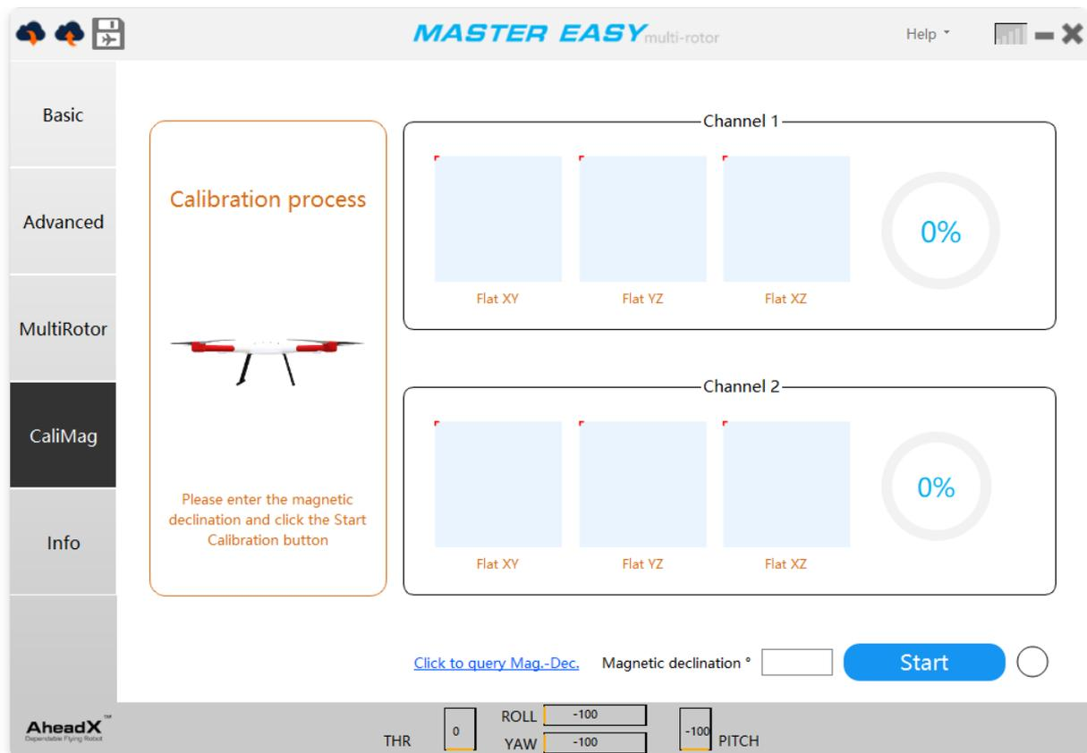
When Taurus 2 performs advanced magnetic compass calibration, it will simultaneously calibrate the internal magnetic compass and satellite compass module of the flight control. After completing the advanced calibration, a pre-takeoff check-magnetic compass status check is required.
