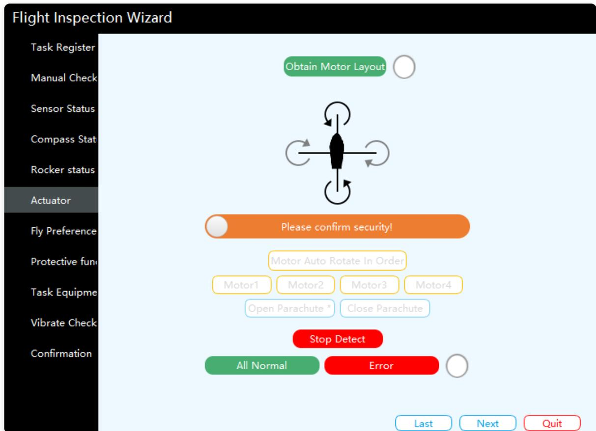
Click the Get Model button, and the current flight layout diagram will be displayed. After confirming the safety of personnel and equipment, drag the slide bar button to the right to start the inspection of the actuator of the motor and umbrella cabin (if included).
