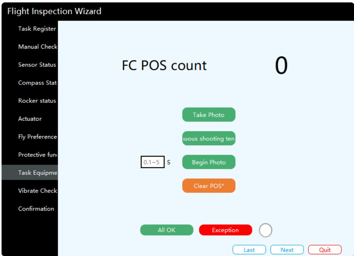
Perform manual photographing to check whether the actual number of camera photographs is consistent with the flight control record value. It is recommended to clear the last POS record data before each operation.
