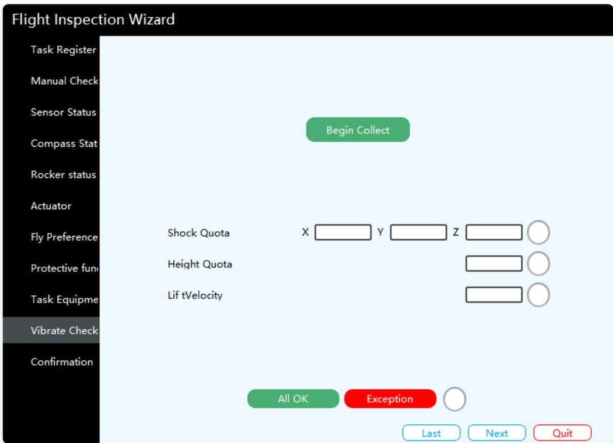
It is used by oil-powered drones to detect engine vibration on the ground. After clicking the Start Collection button, data collection will be performed automatically, and click the End Collection button to end the collection and verify the data.
