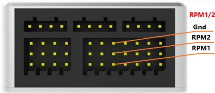
Speed measurement interface, support 2-way speed measurement.
