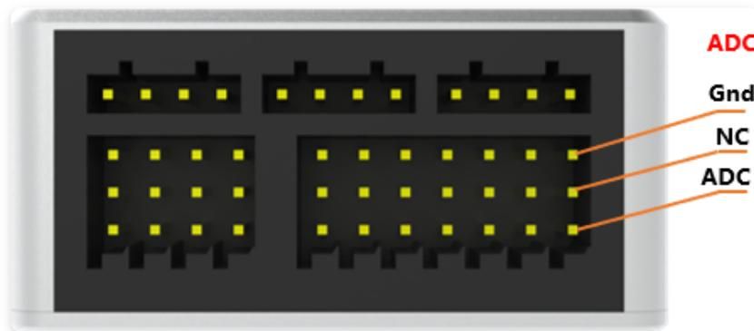
Flight control voltage 3 acquisition interface.
