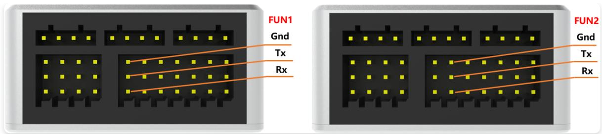
The Rs232 extended serial port can be connected to the AheadX DG3 differential positioning and directional system airborne end, Sirius engine or other devices that conform to the AheadX serial communication protocol.
