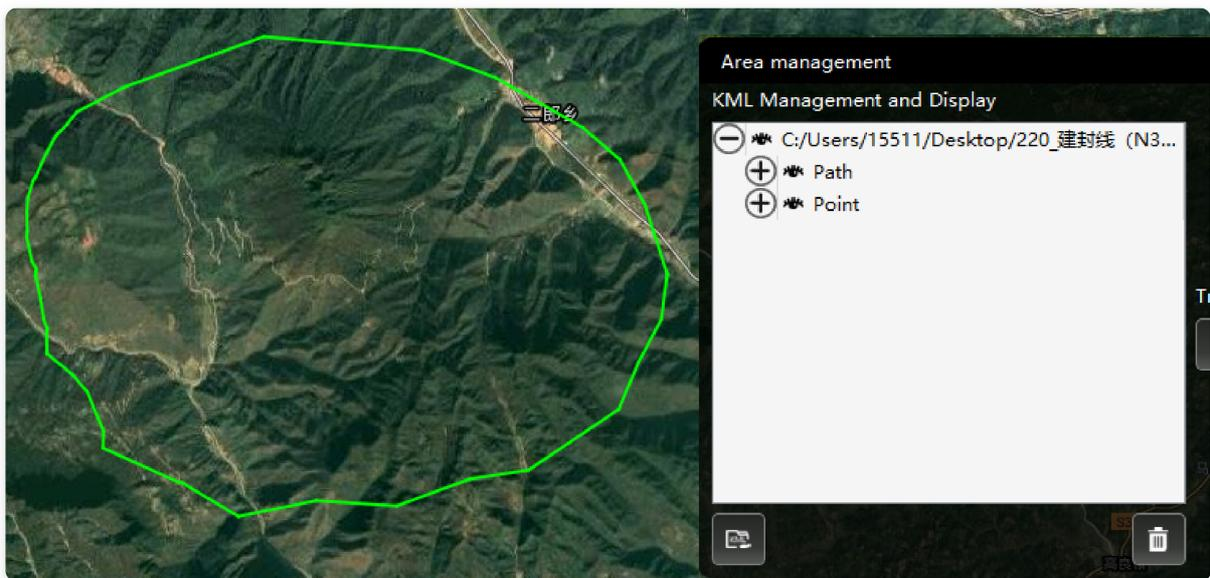
Click the button
