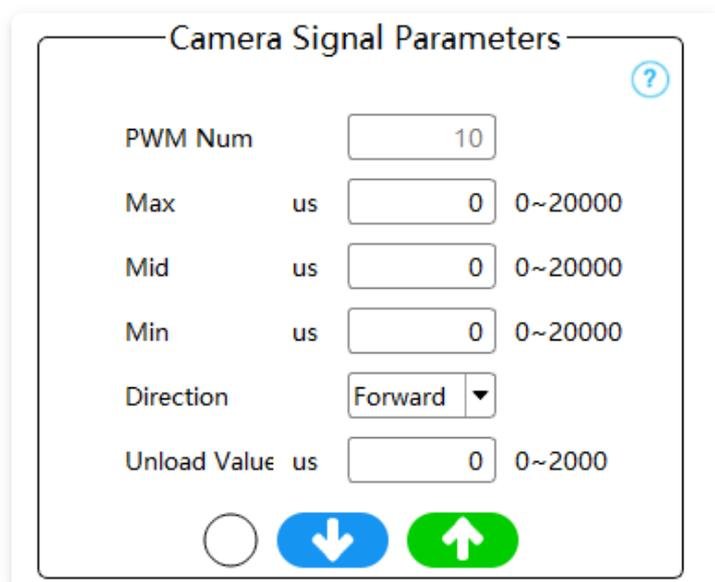
Set the direction to reverse, upload and save the parameters.
