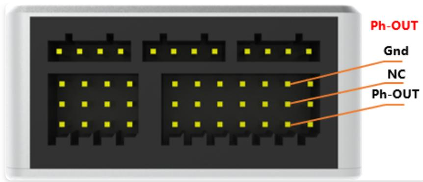
Camera trigger interface, default high level trigger.
