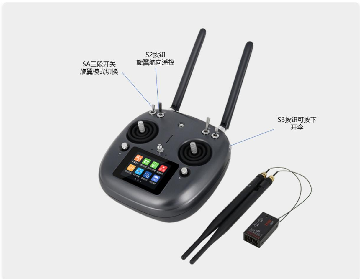
SA: down: rotor attitude remote control; up: rotor attitude position remote control;
