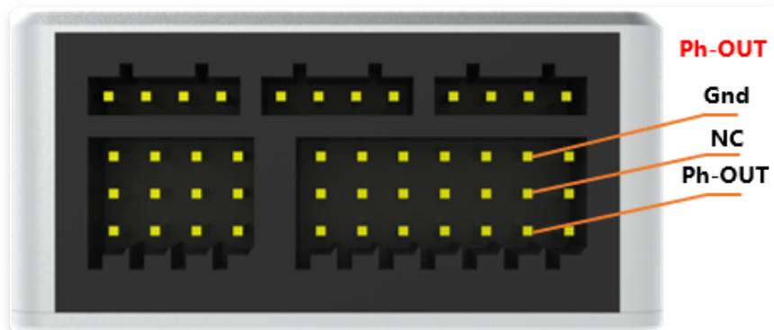
Connect the camera signal line to the Ph-OUT pin. The default is rising edge trigger.
