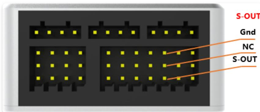
SBUS output interface, can be connected to SBUS flight or mission steering gear.
