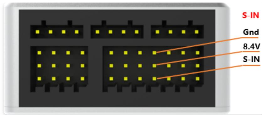
SBUS input interface, connected to the auxiliary joystick receiver.
