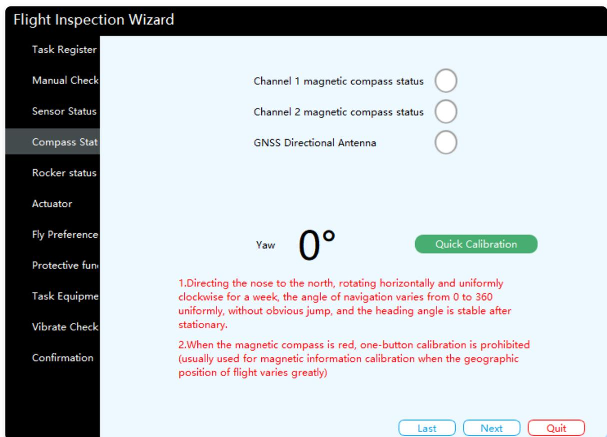
Entering this check interface will automatically refresh the magnetic compass information. If a yellow magnetic reference out of limit prompt appears, you can perform "one-key calibration". If the magnetic compass reports red, please check the interference source first. If there is no interference, please perform the advanced calibration operation of the magnetic compass.
