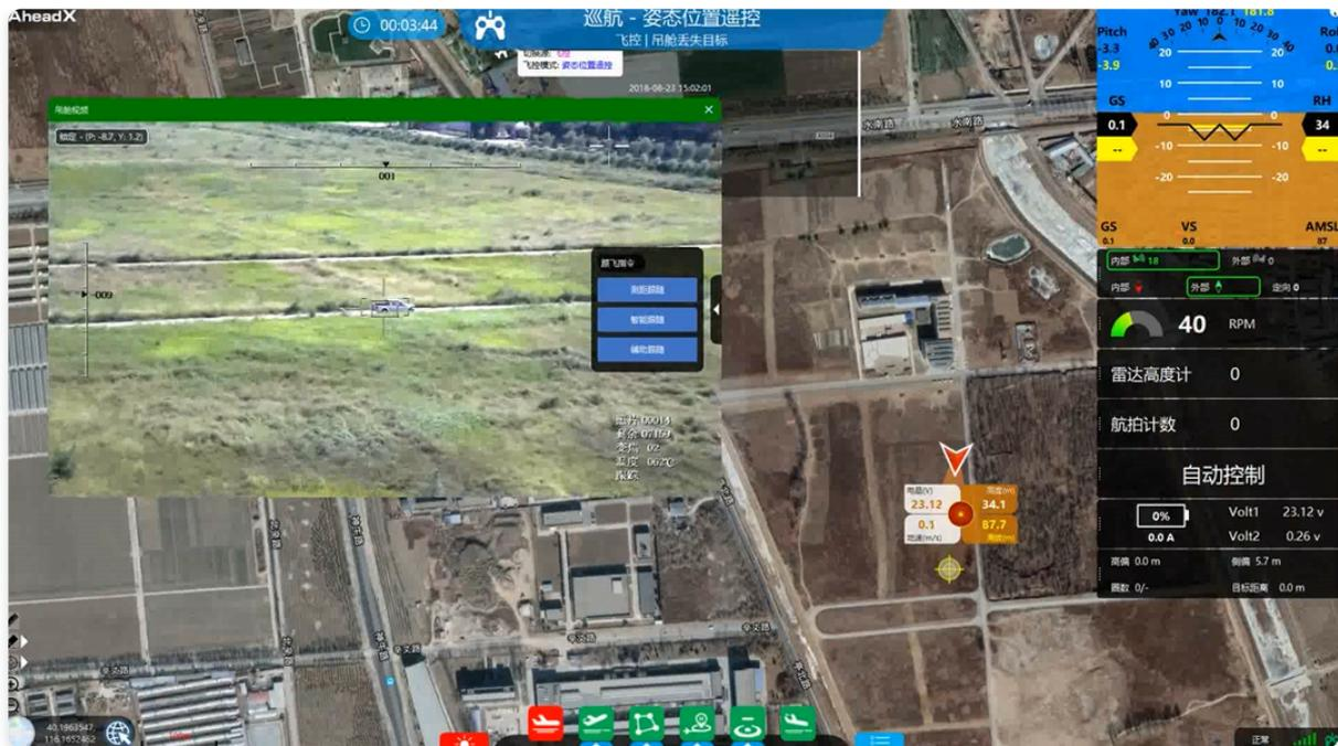
Click the right button of the pod video to call out the pod tracking menu. The multi-rotor pod follows three basic commands.
