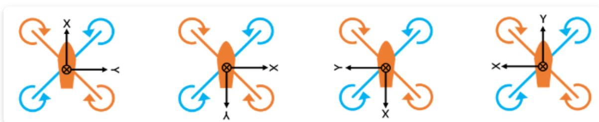
During installation, the silk screen coordinates of the flight control surface shall be consistent with the illustrated coordinates.
