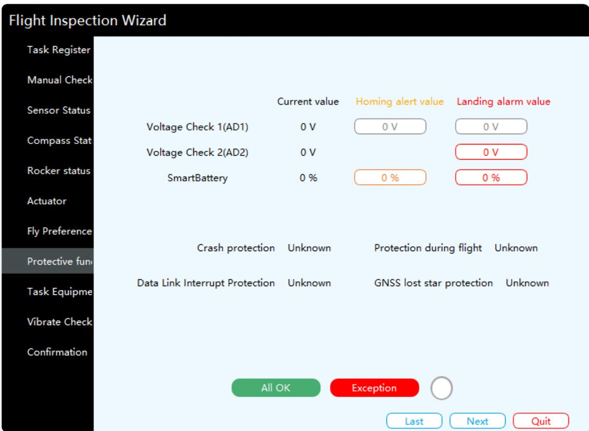
Opening this interface will automatically refresh the current flight control protection parameters. After checking the correctness, click all normal buttons to pass this check. If the protection parameters are set incorrectly, please enter the Master Assistant software for configuration.
