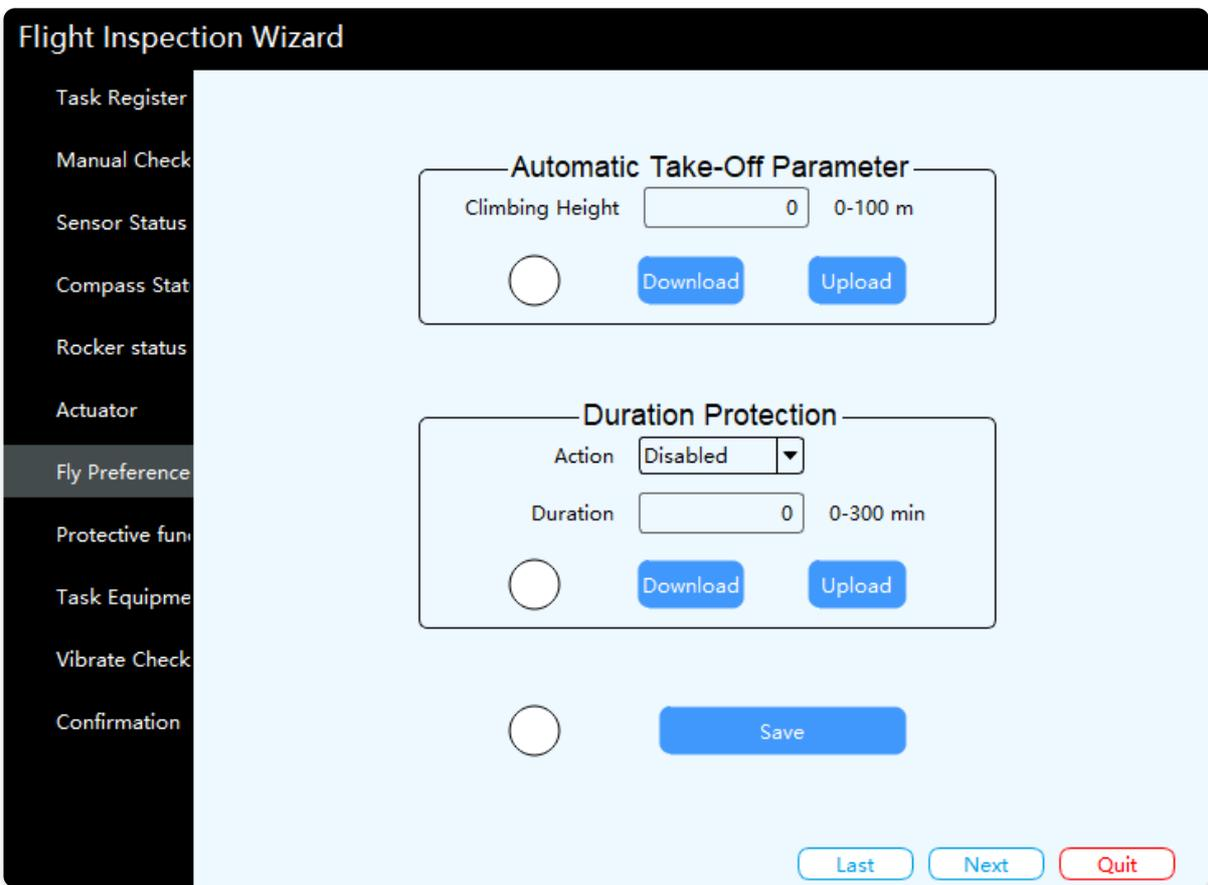
After entering the check page, the parameters will be downloaded automatically. The parameter upload is not saved, only this flight control start takes effect, and it will remain effective after saving.
