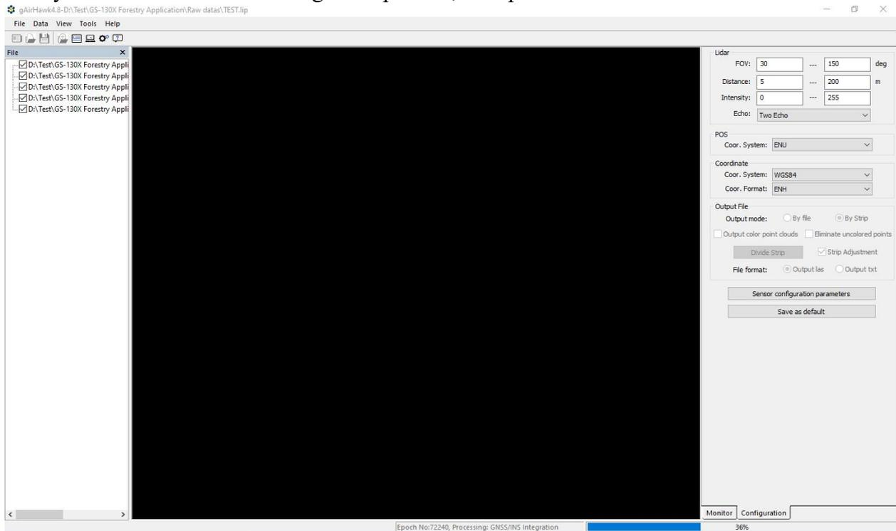
During processing, forward & backward the roller of mouse to zoom in/out, the point clouds display strip by strip.
