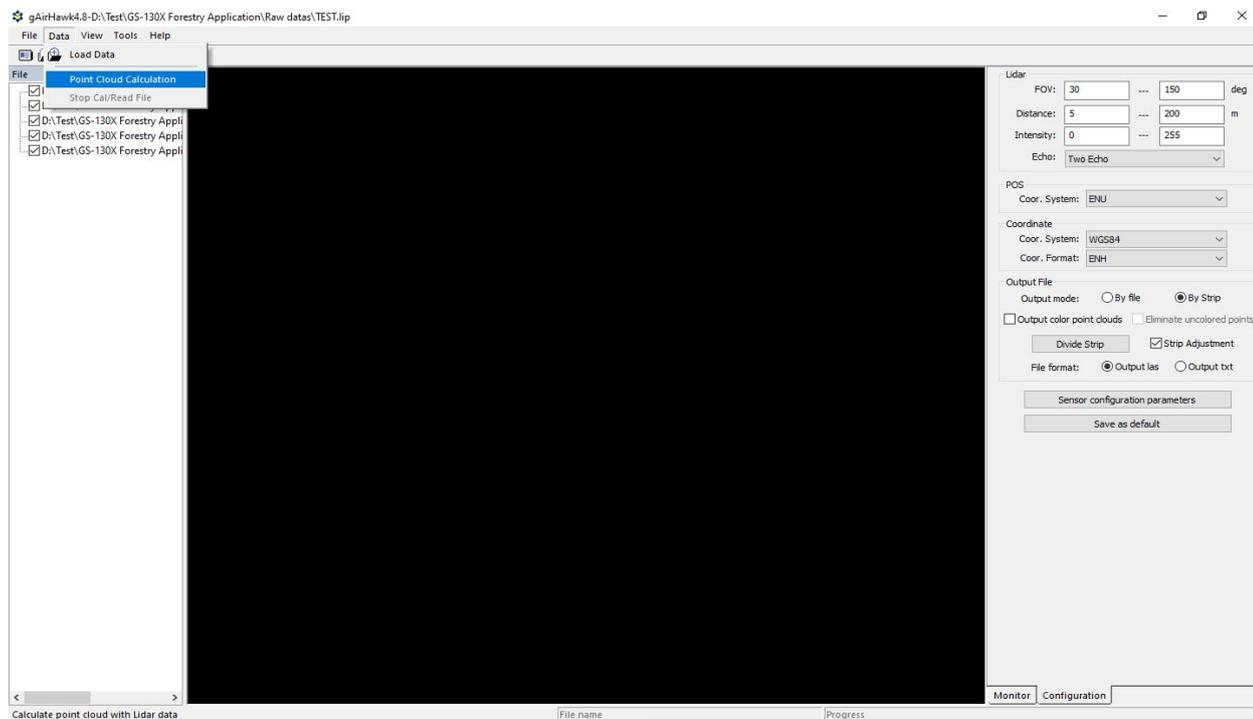
Firstly it does the GNSS/INS integration process, then process the LiDAR data.
