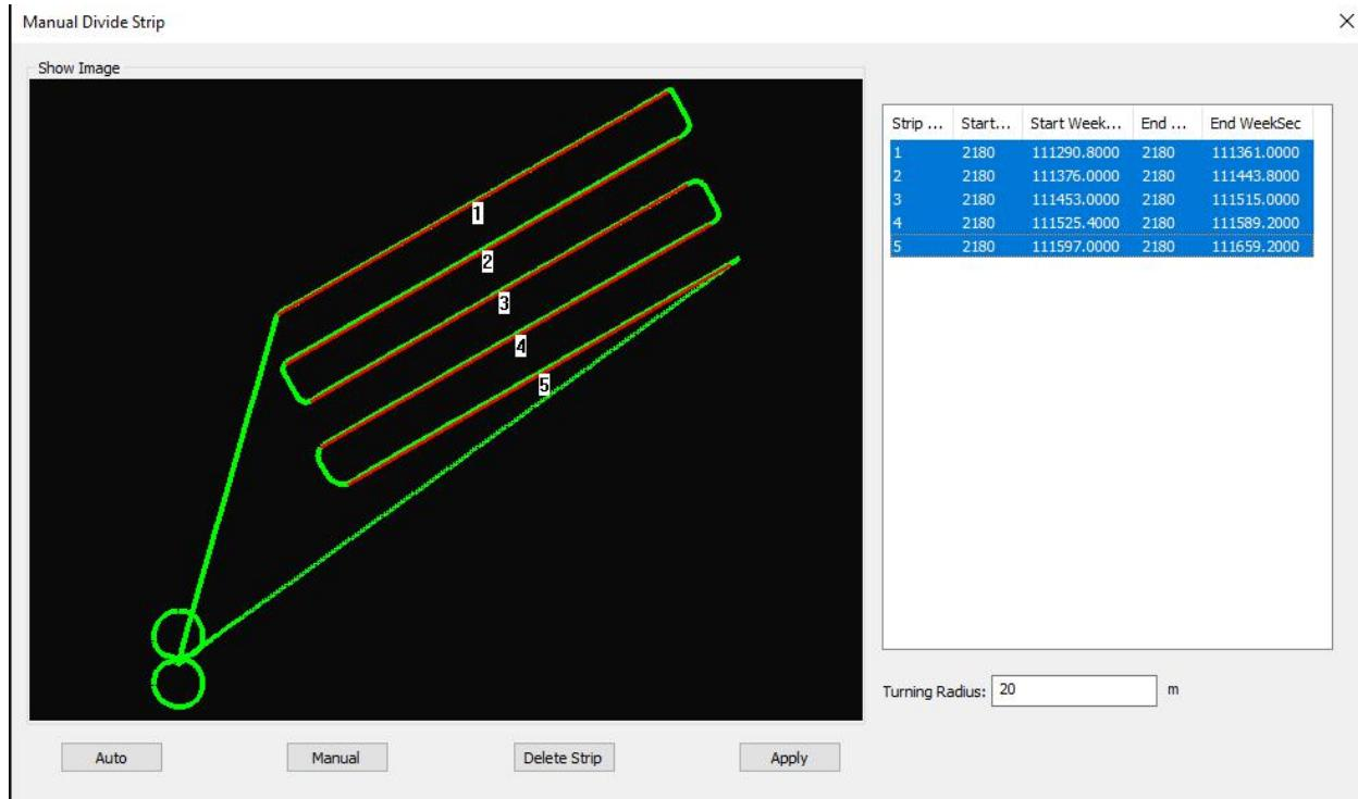
When select Strip Adjustment function, the strips are only selected from North to South (South to North) or from East to West (West to East), but not full strips.
