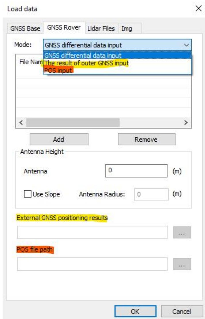
Hereby we only select the GNSS differential data input for **One-Key Process solution**.
