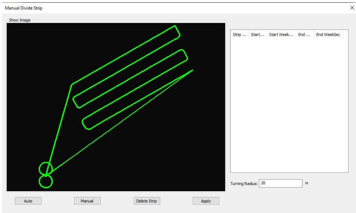
Enter into Manual Divide Strip interface, click the Manual bar to choose the strips (the client could choose the strips according to requirements, and only straight strips are chosen, removed radius parts)
