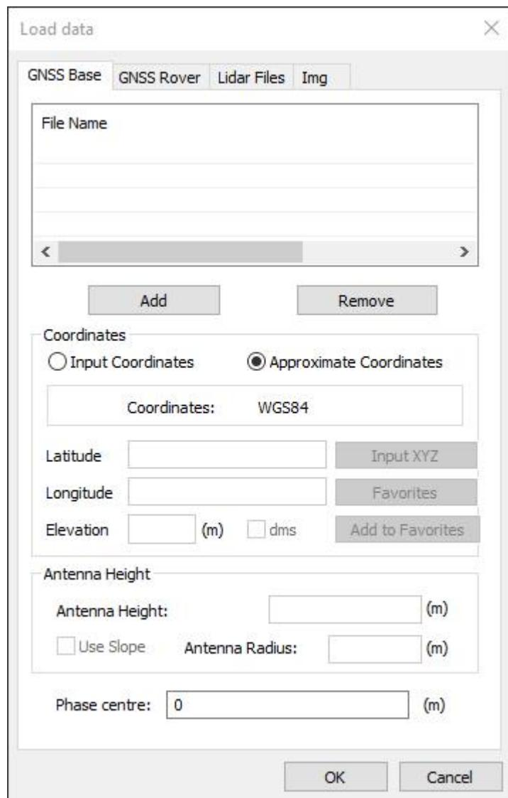
There are GNSS Base bar, GNSS Rover bar, Lidar File bar and Img bar (**Only for the lidar system with Camera**)
