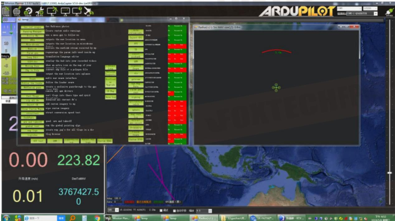
After the above settings are completed, then can perform the outdoor test. When the drone is less than 3m away from the obstacle in gps mode (less than 10m in the fixed height mode), the drone will have a brake action, and the joystick cannot make the drone continue to fly forward.
