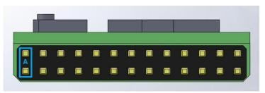
This port supplies power to the TFPro. The TFPro has its own switching power unit so it can be powered from 7-20V. But if you want to share this power with the camera and the video transmitter, we recommend you to power the AP with a 3S lipo since most of the camera and video TX need 12V.
