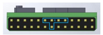
This port is for current sensor, battery voltage sensor and RSSI input.
