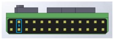
PIN#2 is connected with PIN#1 internal. PIN#15 is the power supply pin for Camera and VideoTX.
