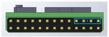
This port is used for the optional telemetry data radio.
